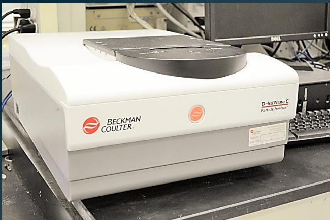
Beckman Coulter, Delsa Nano, Dynamic light scattering particle size analyzer
