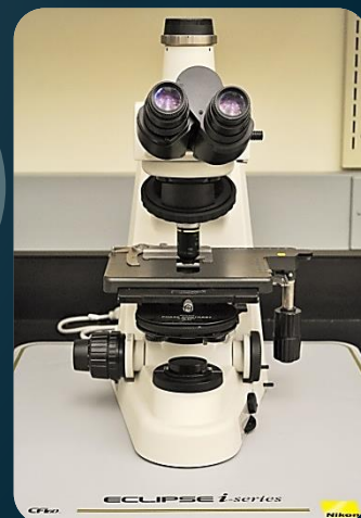
Nikon Eclipse 50i Polarized Light Microscope
