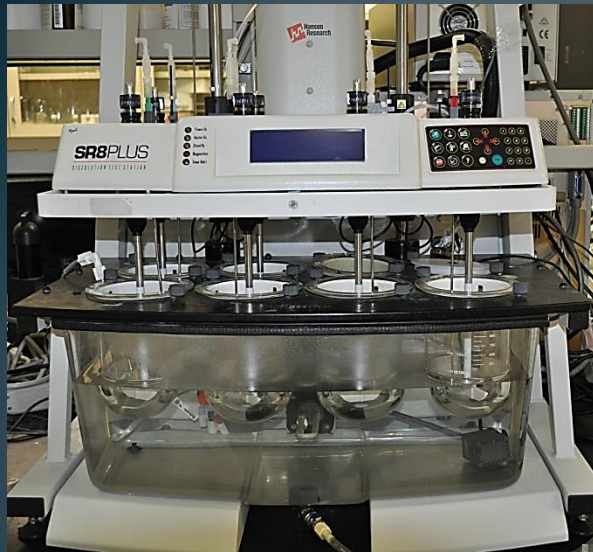
SR8 Plus Dissolution Station, Distek Dissolution Apparatus
