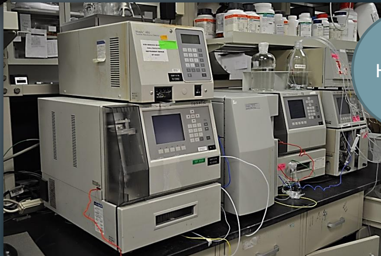
Agilent 1100 series HPLC (2), Waters Corporation HPLC (5)
