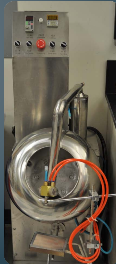
Shanghai Tiangfeng , Waternut Type Tablet Film Coating machine
