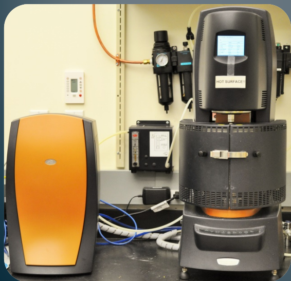
TA Instruments, Discovery HR-2 Hybrid Rheometer
