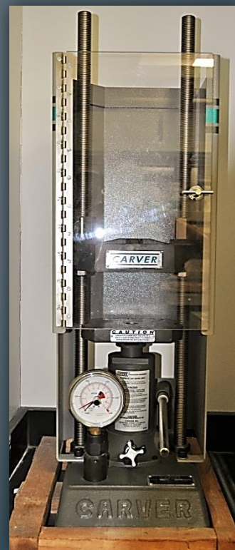
Carver Tablet Press, Single station Model C
